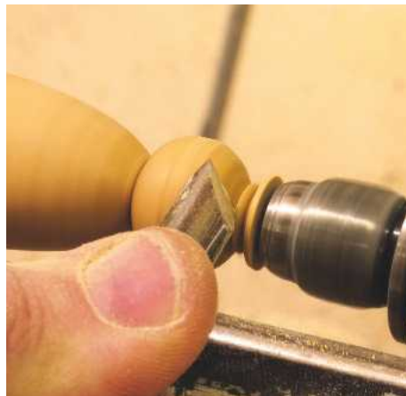
▲ Pic.32 The little bead on the end is turned with the skew. When you sand the handle make sure that you don't soften all the crisp detail that you have turned so far
